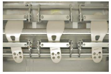
Fleximeter for long life test on thermoplastic soles
