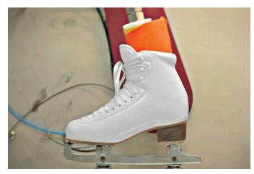
Flex testing machine, for long life test and stiffness measurements
