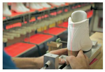
Laser control, to check if the sole and the upper are aligned
